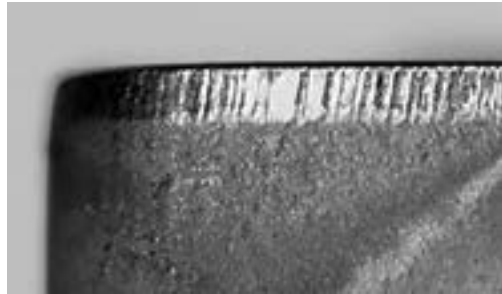
Abrasion on flank, normal wear after a certain machining time.
