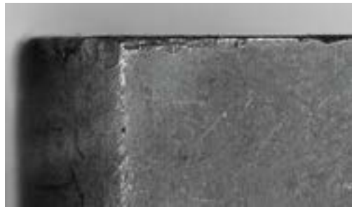
Through excessive mechanical stress at the cutting edge fracture and chipping can occur.
